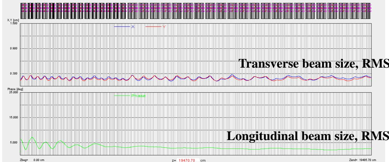
using TRACK code with 100k particles/charge state
