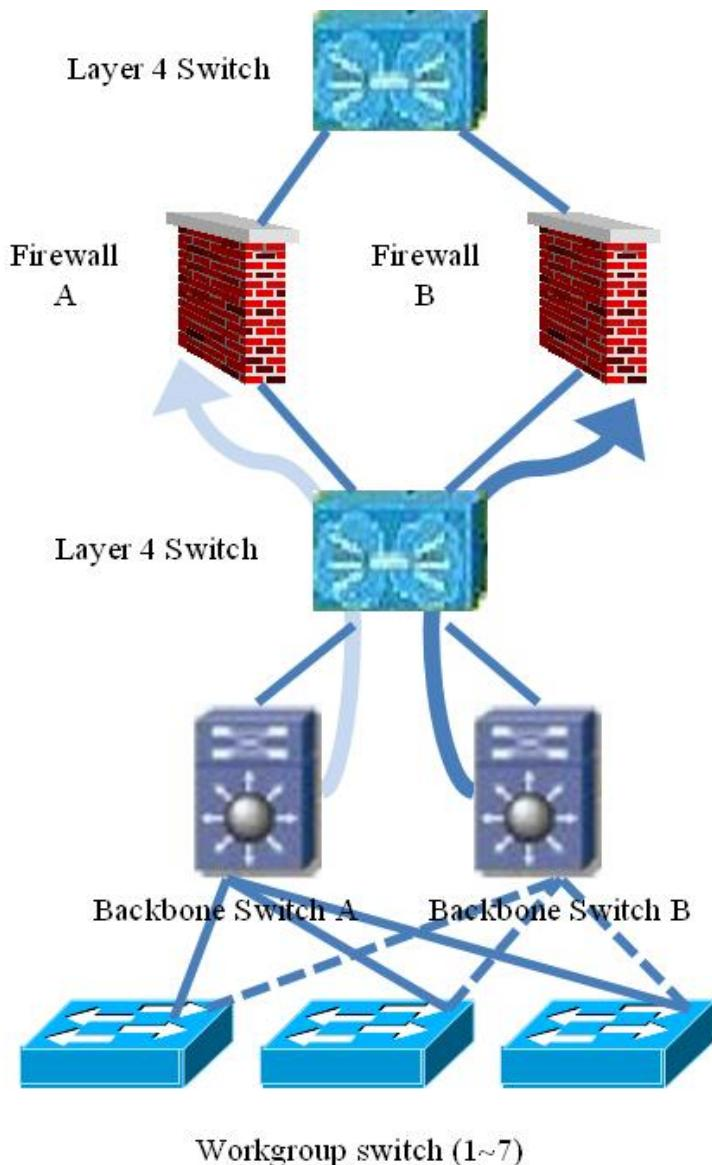
Conceptual drawing for network failure
