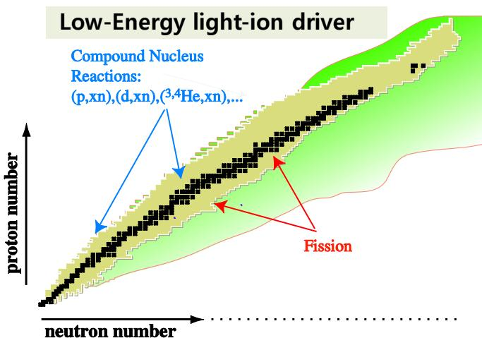
**Fission reaction is best way to produce neutron-rich RIs, especially medium-mass region.**
