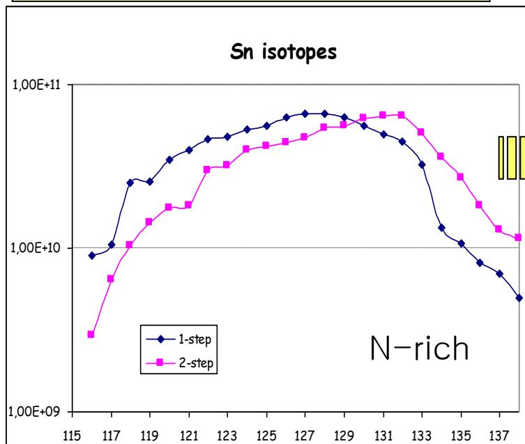
Beam intensities evaluated considering release, ionization and reacceleration efficiencies
