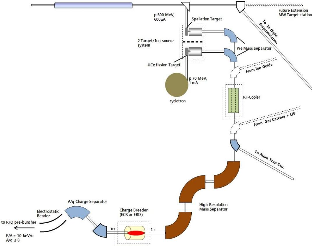
ISOL RIB Extraction system layout
