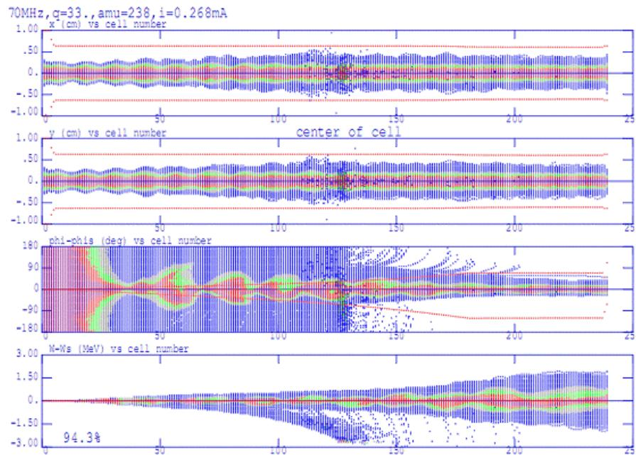
Kinetic energy and transmission characteristics of uranium beams in RFQ
