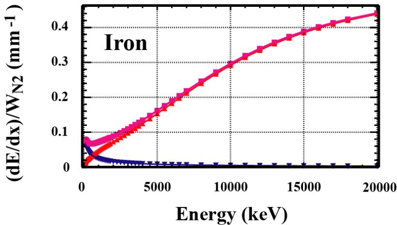
$$(dE/dx)_{\text{total}} = (dE/dx)_{\text{electronic}} + (dE/dx)_{\text{nuclear}}$$
