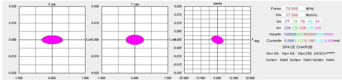
$$\begin{aligned}\epsilon_{nx, \text{ rms}} &= 0.30 \text{ mm mrad} \\ \epsilon_{ny, \text{ rms}} &= 0.28 \text{ mm mrad} \\ \epsilon_{nz, \text{ rms}} &= 0.87 \text{ keV/u ns}\end{aligned}$$
