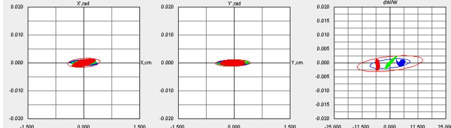
❖ Synchronous phase  $\phi_s$  is set to be  $-30^\circ$
