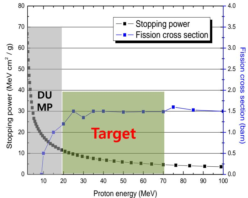
Fission cross-section vs. stopping power on proton
