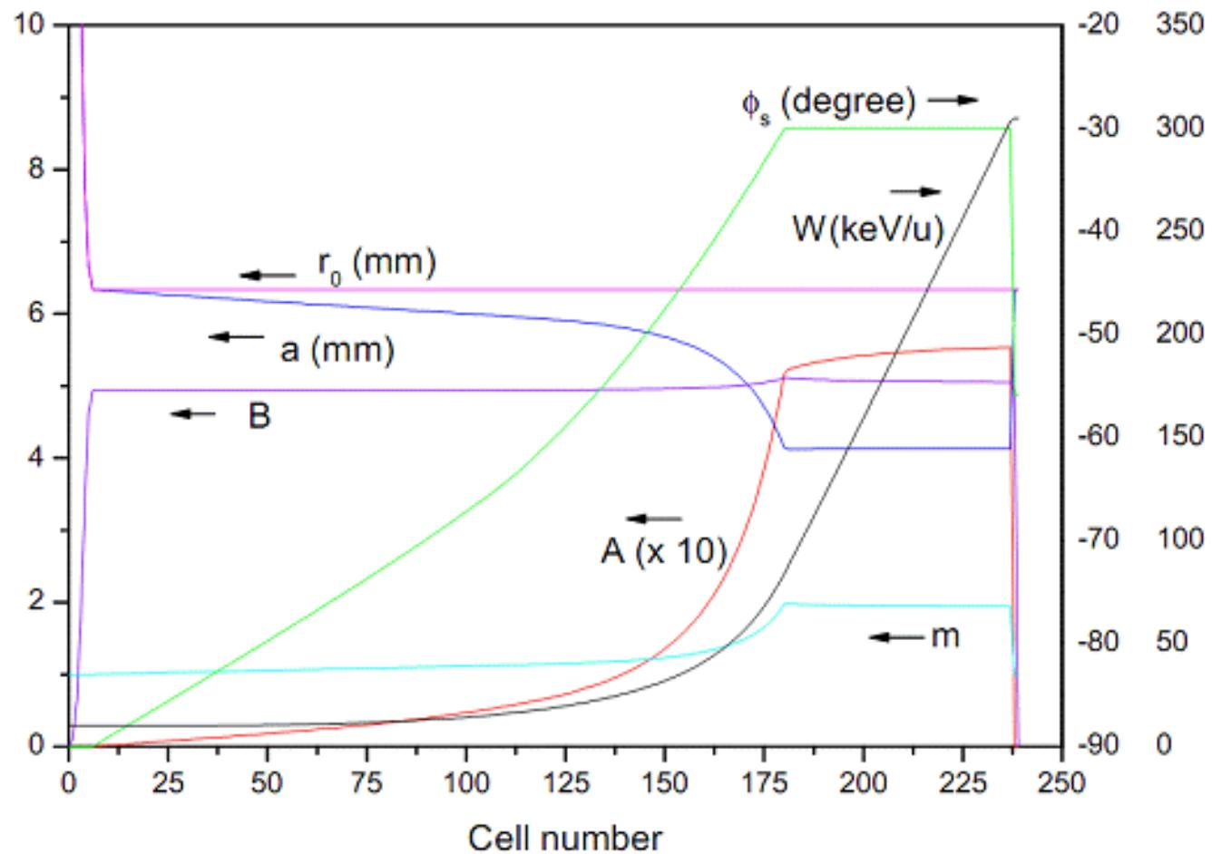
a(aperture radius),  $r_0$  (average aperture radius), m(modulation),
