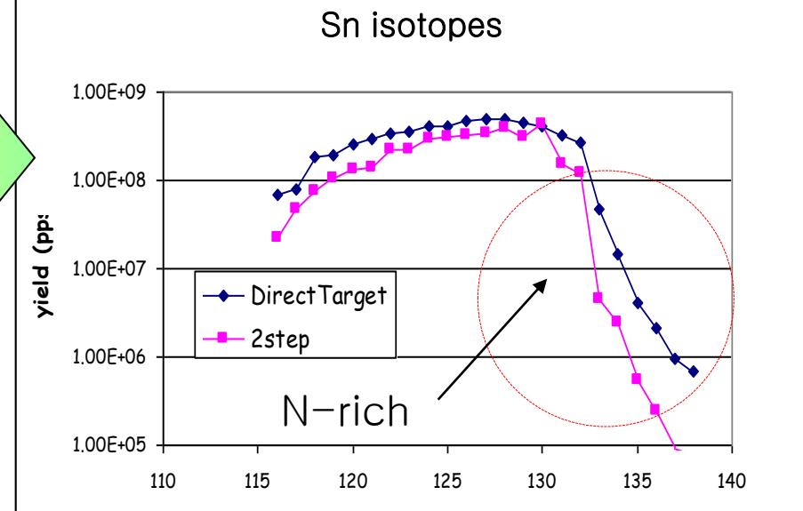
Direct target have advantages to provide neutron-rich beams
